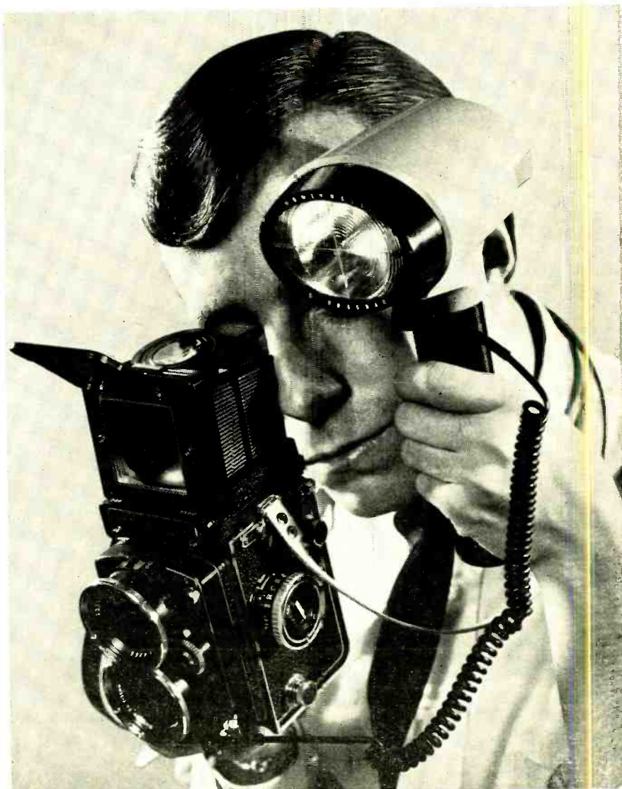
Smaller still: Circuits for this photocell-regulated flash, Honeywell's Auto-Strobonar 660, have been packed into a smaller but similar automatic strobe, the 440, for shoe mounting (see page 42). New techniques simplify miniaturization.
