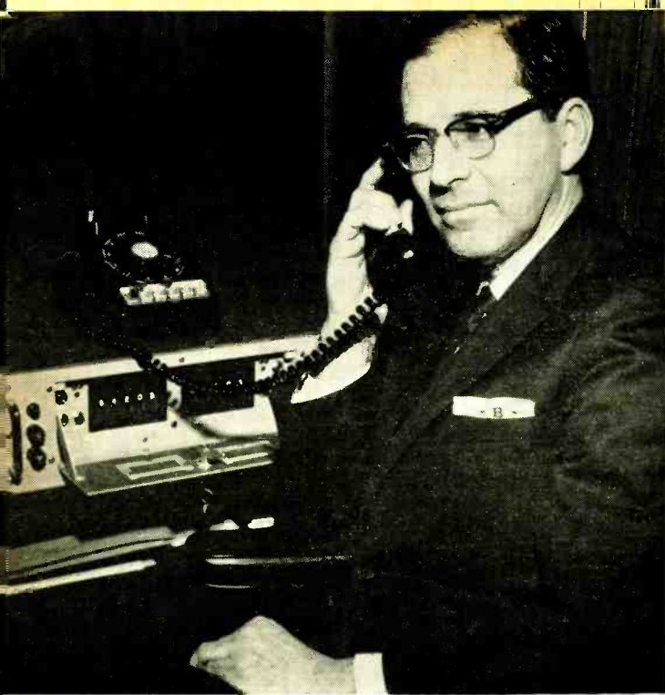
When telephone bugging is suspected, this "scrambler" assures private conversation. Voice is electronically coded and decoded at sender's and receiver's station.
