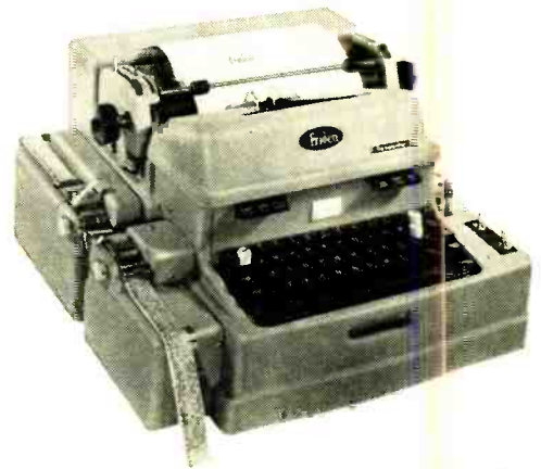
Fig. 1—High-speed Friden typewriter uses punched tape.
