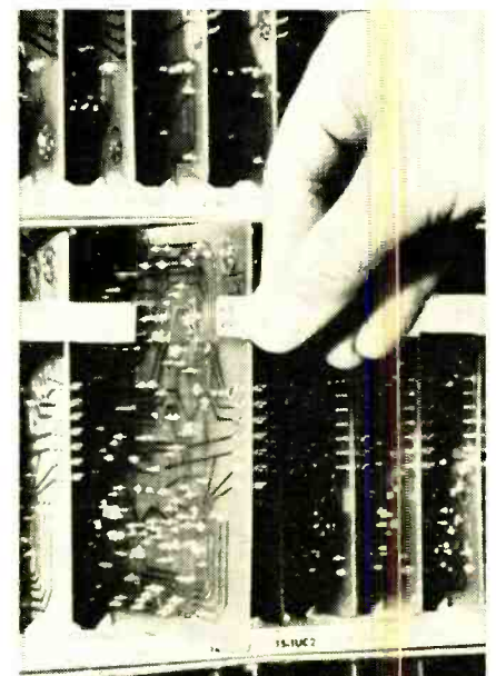
▲ Fig. 3—Plug-in modules used in the Mark Century control system (Fig. 2).
