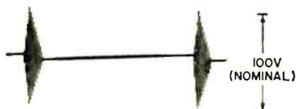
Fig. 5—Amplified burst at t.p. L (above) may appear with a gradual sawtooth voltage, due to integrating effect of probe.
